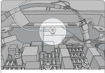
**Step 8:** Attach the grounding ring terminal and reinstall the ground screw.
