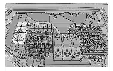
**Step 7:** Use zip ties to secure the **HRN-CE10A2** and **HRN-CM24Y1** harnesses then place the wires inside and replace the panel cover.
