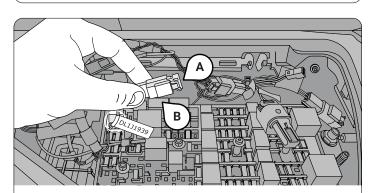
Step 11: Locate the OEM gray 2-pin Deutsch connector (DTM04) with label DL1J1939. Where EOL resistor is present, remove the EOL resistor A from receptacle B.
