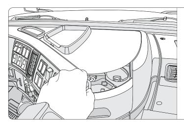
**Step 1:** Remove the fuse box panel — located under the center console between the driver and passenger seat. Use the two T25 torx head screws to remove the panel.
