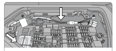
Step 13: Secure the GO device and harnesses with zip ties.
