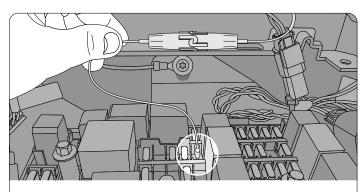
**Step 10:** Insert the fused spade terminal into the fuse holder side that provides 12 volts constantly.
