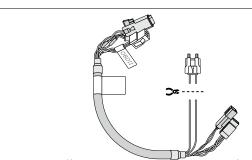
Step 3: Cut off the white spade power connector from the HRN-CE10A2 harness.
