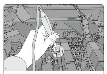
**Step 9:** Locate an empty or spare fuse slot, and test which side of the fuse holder provides 12 volts constantly. Try to use fuse slot #71, if available.
