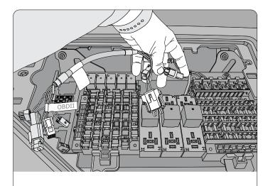
**Step 3:** Connect the **HRN-CE10A2** to the vehicle side where the End of Line resistor was removed from.
