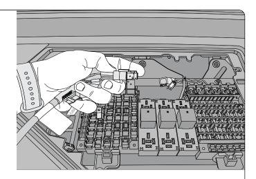
**Step 2:** Locate the OEM 2 pin gray connector (J1939) with the End of Line resistor. Remove the End of Line resistor from the vehicle connector, then immediately insert the End of Line resistor into the mating connector of the **HRN-CE10A2** harness.
