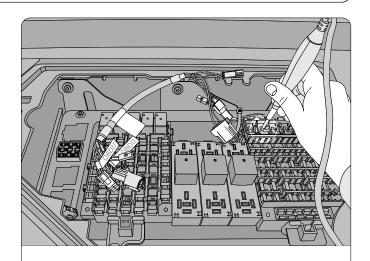
**Step 4:** Plug in the **HRN-CE10A2** 2-pin power connector into the tested and verified power slot.
