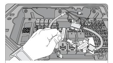
Step 6: Connect the 6-pin white Molex connector of the HRN-CM24Y1 harness labeled OBDII to the 6-pin white Molex connector on the HRN-CE10A2 harness labeled OBDII.
