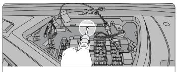
Step 6: Locate and remove the T-25 grounding screw.
