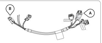
Step 12: Insert the gray Y connector of the HRN-CE10A2 harness and connect the components labeled A and B (i.e. A to A and B to B) — as indicated in the image above and in step 4.
