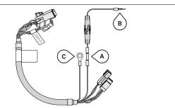
Step 4: Connect the fuse-holder set to the red power cable A.
